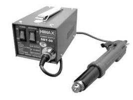
Fulfill the preset depth, auto stop and return. SB-400C & SBT-50 is the best tool for preventing break of screw tap. The machine can auto sense the excessive load between the screw tap and screw hole and return to prevent break of screw tap Whether for a stop hole or through hole, it can fulfill the preset depth then auto return and exit to improve the work efficiency. Besides that, the depth of screw tap can also be freely adjusted.
